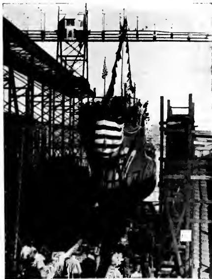
A bow view of the torpedo boat destroyer "Shaw" sliding down the ways at Mare Island.
